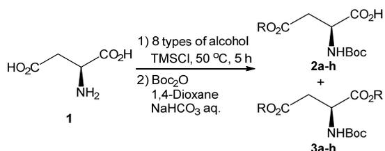
**Figure 1:** Selective esterification using TMSCl as an acid catalyst precursor.
